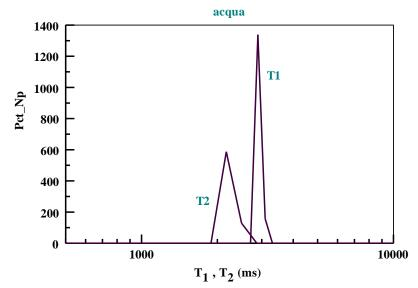
The relaxation times are plotted on the x-axis in log-scale. On the y-axis the percentual value of the normalized signal density (signal normalization, the areas of the curve are the same) is represented. (Using the Sig\_Np, the area of the curve indicates the absolute acquired signal).
