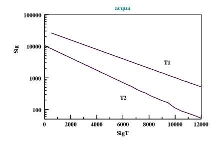
Sig indicates the intensity of the signal in arbitrary units. SigT represents the time t in ms. The intercept to the y-axis (SigT = 0) indicates the total NMR signal, proportional to the water amount in the glass tube. In the semi-logarithmic scale, the linear trend of the curves suggests a mono-exponential decay, expected for a sample in which all the <sup>1</sup>H nuclei are affected by the same chemical-physical environment.
